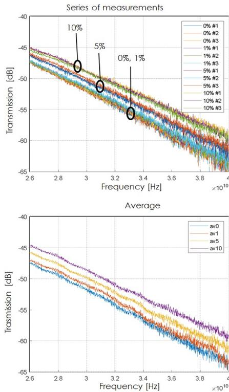
**Fig. 3.** Top panel: Transmission coefficient in dB for a sequence of measurement with isotonic solution and different concentration of sugar. Bottom panel: Average of transmission coefficient in dB computed from the three consecutive measurements with identical sugar concentration. The four curves refer to the following cases: no sugar, 1%, 5% and 10% sugar dissolved in the isotonic solution.
