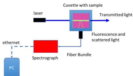
**Fig. 4.** Overview of the measurement setup based on the LIF spectroscopy in the visible band.
