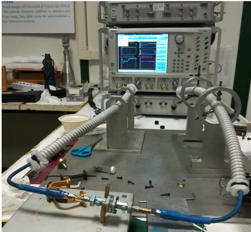
**Fig. 2.** Measurement setup consisting of a VNA (in the background) and input/output coaxial cables connected to the coaxial line - waveguide transitions and to the sample's holder (in the foreground).
