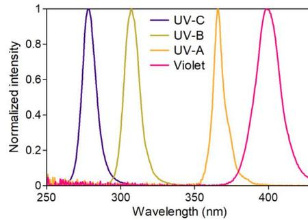
**Fig. 1.** Normalized emission spectra of the LEDs employed in the illumination of the virus stock. UV-C (278 nm), UV-B (308 nm), UV-A (366 nm), Violet (405 nm).
